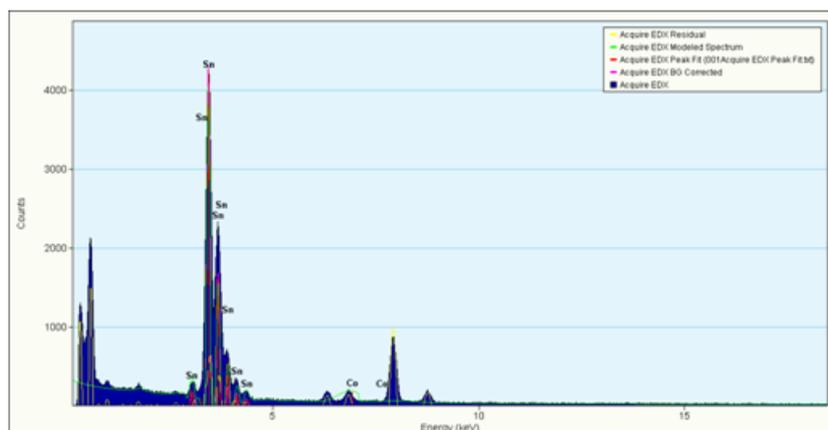
**Fig. 4** EDAX picture of 2% Co doped SnO<sub>2</sub> nanoparticles
