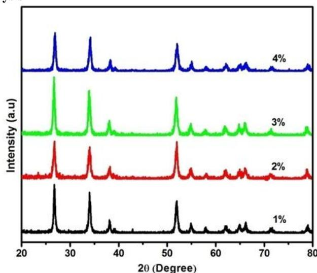
Fig. 2 XRD patterns of Sn<sub>(1-x)</sub>Co<sub>x</sub>O<sub>2</sub> (0.01 ≥ X ≤ 0.04) nanoparticles
