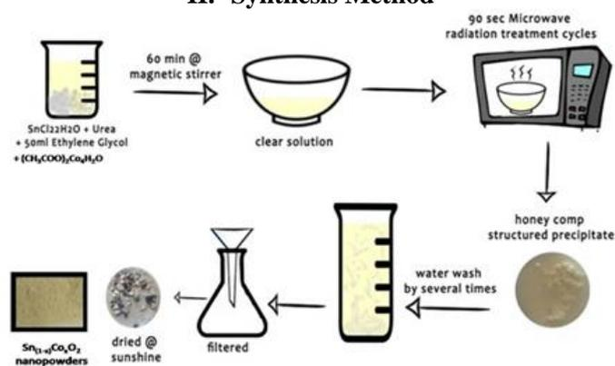
Fig. 1 Synthesis flow chart of Co doped SnO<sub>2</sub> nano particles
