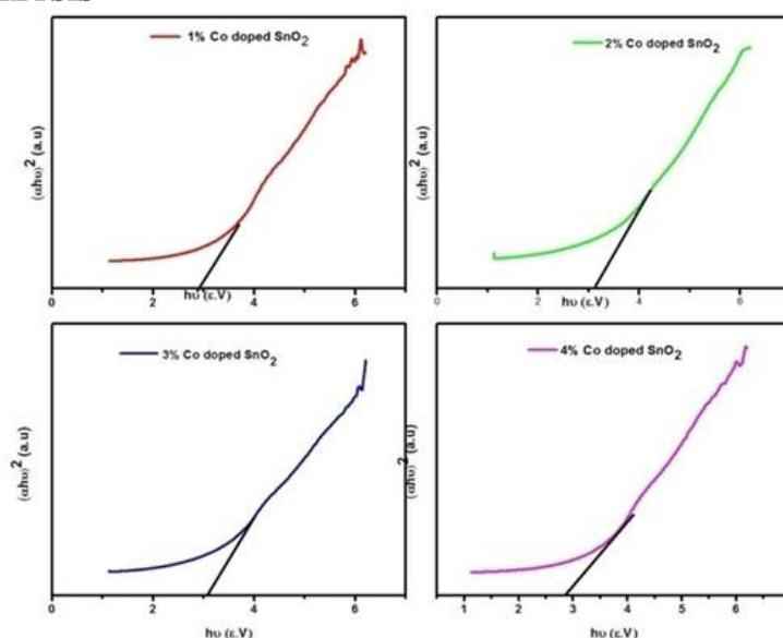
Fig. 7 Tau plot of Co doped SnO<sub>2</sub> nano particles
