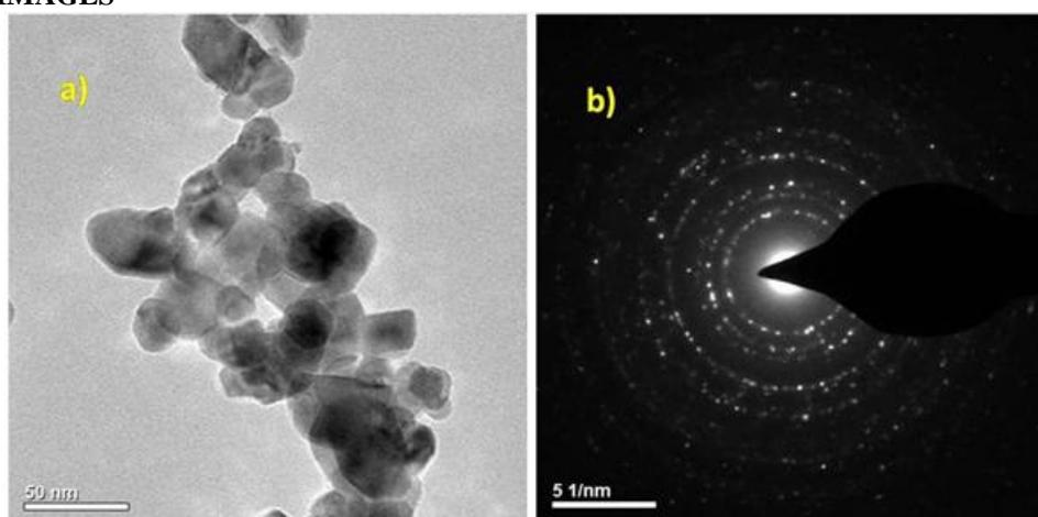
**Fig. 5** (a, b) TEM Image & SAED pattern of 4% Co doped SnO<sub>2</sub> nanoparticles
