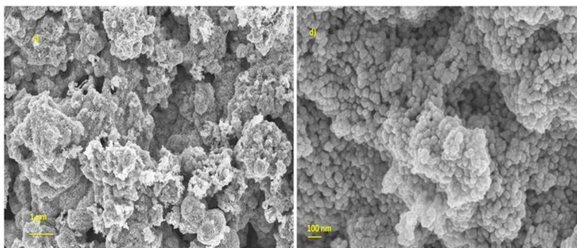
**Fig. 3** (c, d) SEM images of 3% Co doped SnO<sub>2</sub> nanoparticles
