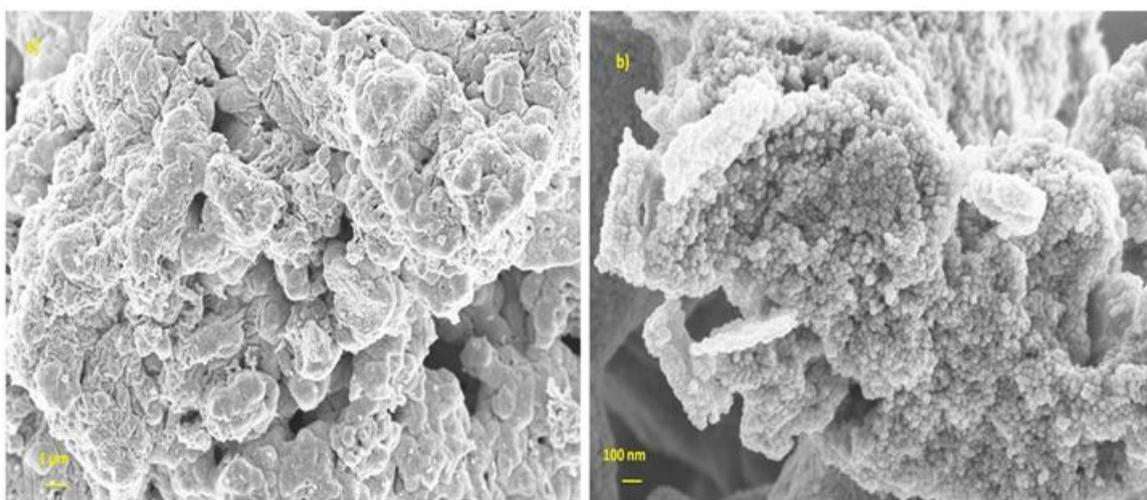
**Fig. 3** (a, b) SEM images of 2% Co doped SnO<sub>2</sub> nanoparticles
